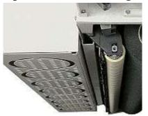
220109 Punched work-top and conveyor belt preset for vacuum device N. 1 (for 2 internal working stations)
